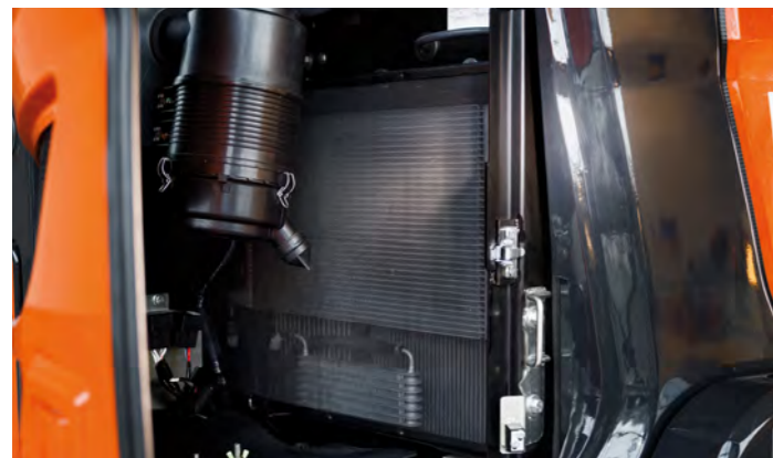
The radiator is easily accessible for cleaning.
