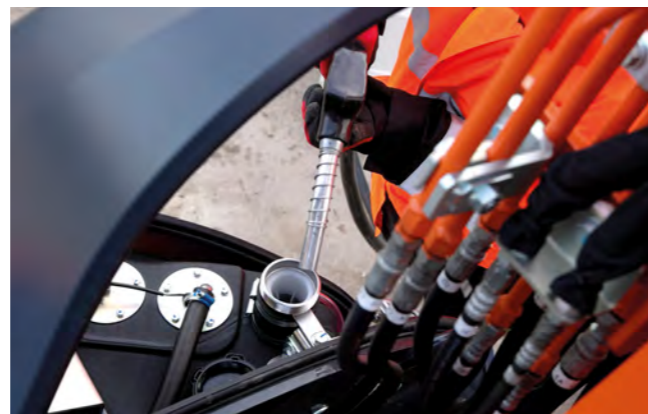
The fuel tank has also been repositioned to make it easier and safer to refill.
