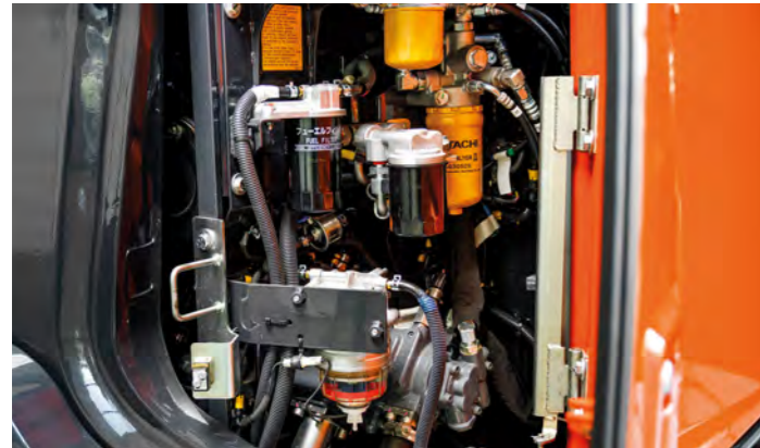
Convenience access to all filters in one compartment.
