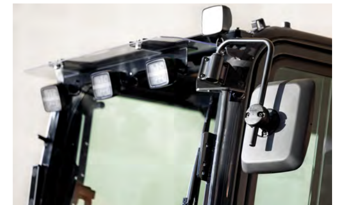
Relocated boom and cab lights improve visibility in challenging conditions.
