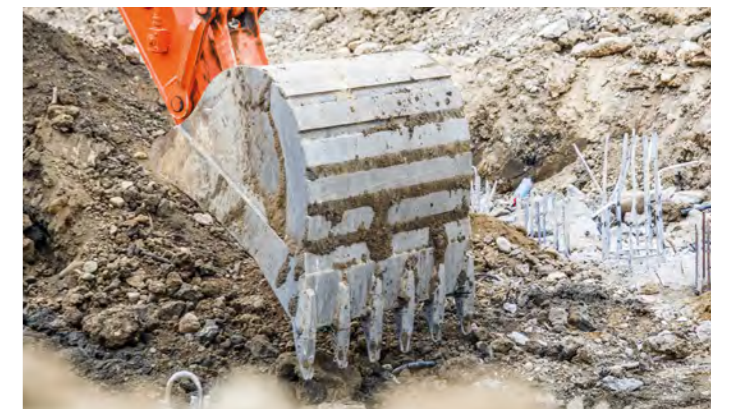
Hitachi GET include self-sharpening teeth and reliable adapters to ensure a precise fit.
