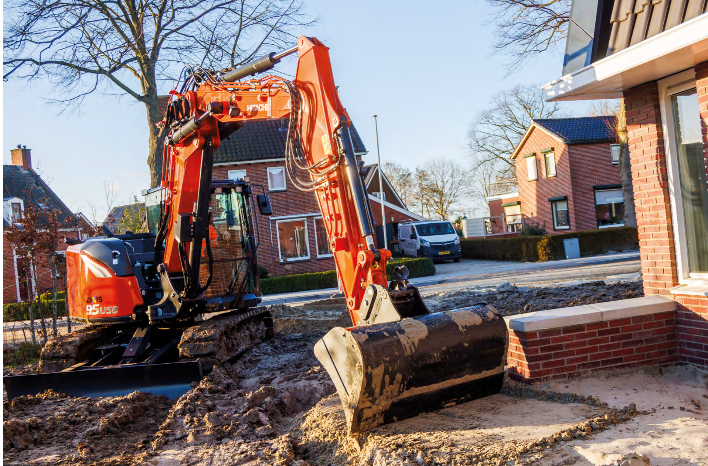
Short distance between the bucket and blade enhances efficiency and safety.
