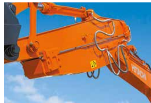
The sliding arm extends the working range of the ZX135US-6.
