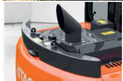
The small additional counterweight is easy to handle and increases stability.
