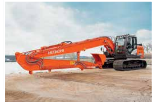
The design of the front attachment allows for easy transportation.
