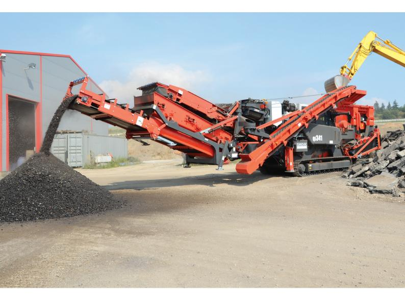
Built utilising Sandvik's market leading Prisec<sup>TM</sup> technology, the QI341 is the most versatile, compact mobile impactor in the market today. Capable of operating in primary and secondary applications, it has been designed with productivity, mobility, minimal environmental impact and user friendliness at its core.
