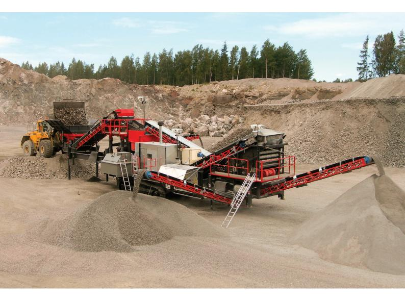
The UH640 is a flexible, highly productive secondary cone crusher that is able to produce finished sized products thanks to an integral product screen and closed circuit operation.
