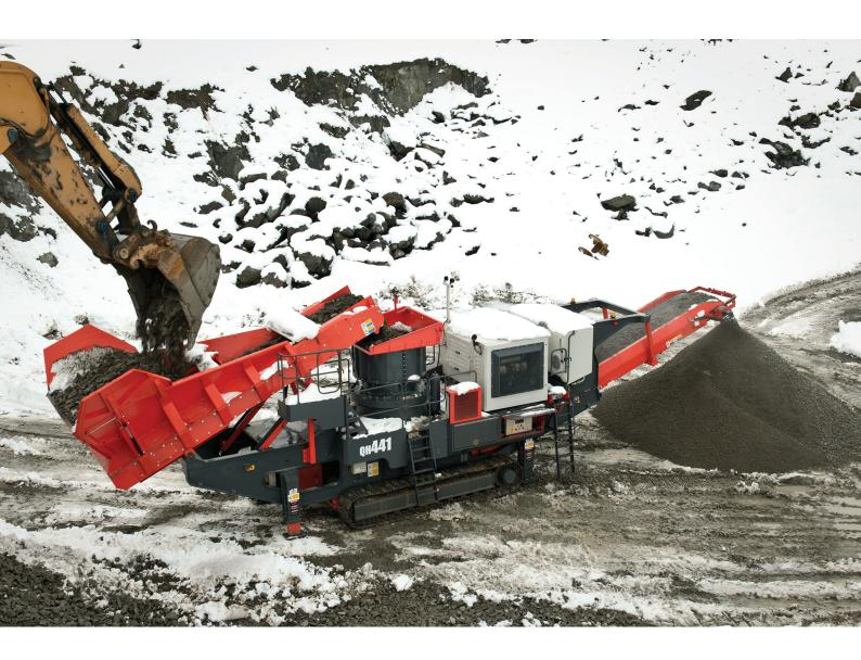
The QH441 is a tracked, self contained cone crusher with an on board diesel engine.
