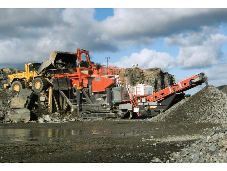
The intelligent UJ540 tracked jaw crusher mounts the highly productive Sandvik CJ612 jaw, on a full tracked chassis but with an electric crusher drive. The CJ612 crusher is a single toggle  $1200 \times 1100$  mm (48 x 44") jaw crusher, which has been designed for high productivity, low energy consumption and automated process control.
